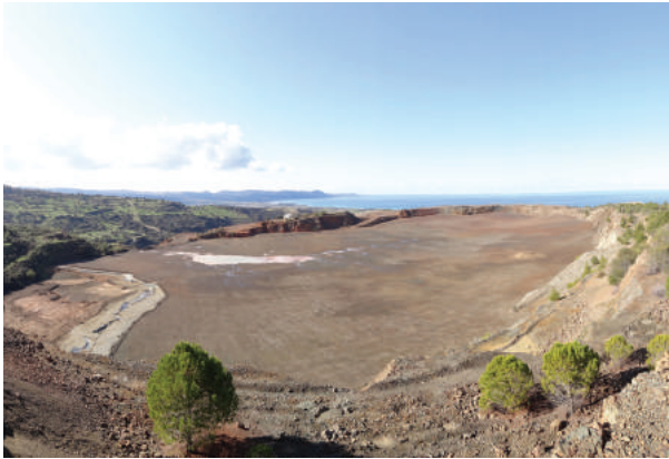
The crater after being filled with 12 million cubic metres of tailings and other excavated materials
