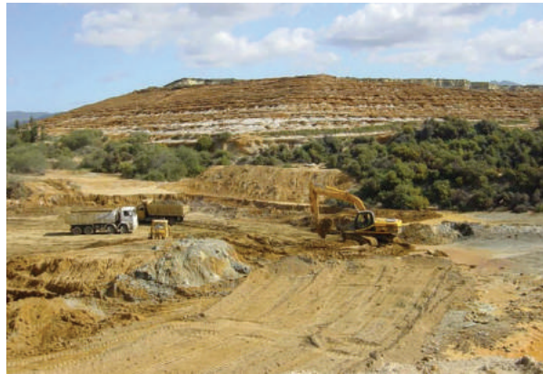
Mount of tailings - 250.000 sq.m, height 35m, volume 4,5 million cubic metres
